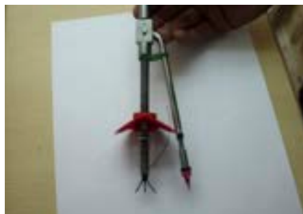
E-Compass A Compass that Forms Ellipses
