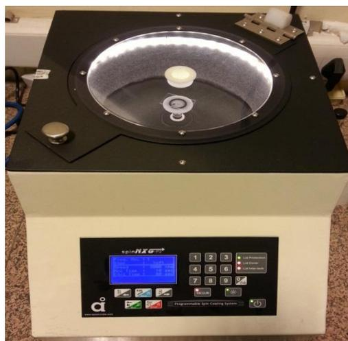
Spin coating unit used for thin film deposition.
