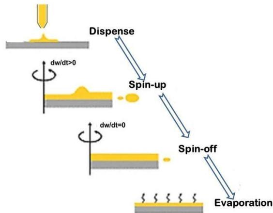
**Fig. 2.2:** Schematic representation of the spin coating process.
