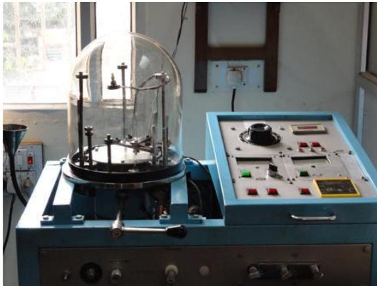
Thermal evaporation unit for depositing thin films.
