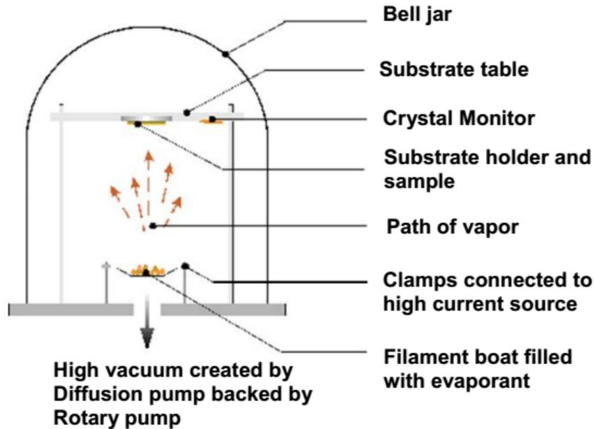
Schematic representation of thin film fabrication via thermal evaporation of the material in vacuum chamber.
