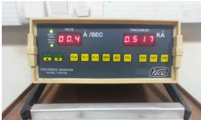
Device for insitu film thickness measurement.
