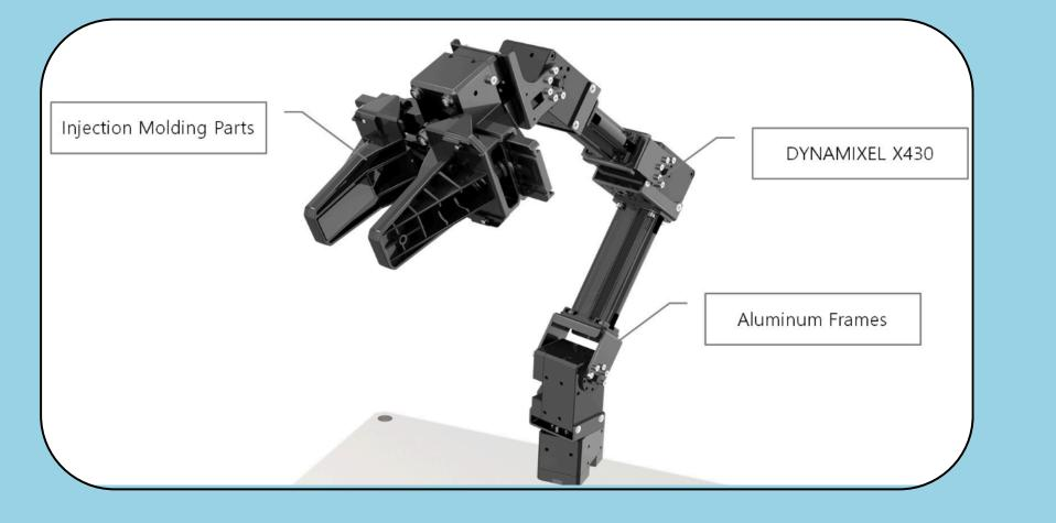
Developed by ROBOTIS, the OpenManipulatorX is an open-source robotic manipulator with several joints for diverse movements, intended for use in research and education. It is managed by a microcontroller with many communication interfaces, under the direction of a kinematic system and dynamics considerations. To ensure that the algorithm is validated before being physically implemented, the manipulator is tested in the Gazebo simulation environment.
